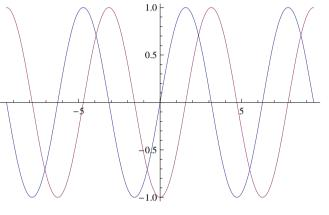
The curve in blue is the same as the sine wave plotted above, the curve in purple is 90 degrees out of phase of the blue curve. This means that when the blue curve reaches its maximum value, the red curve is at zero.
