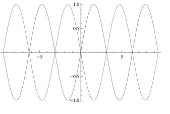
Look carefully at the yellowish line that represents the sum of the waves. Notice that when the two waves are 180 degrees out of phase, they completely destroy each other, producing no light or sound at all. When we study diffraction patterns, we are observing how two or more waves can combine to produce more intense waves, or can combine to completely null themselves out.
