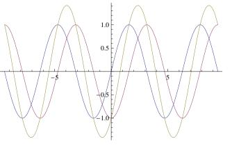
Let's look at the above curve a little more closely. We can see that there are locations where the waves add to produce greater intensity (a brighter light or greater sound), and there are places where the waves cancel out to produce no intensity at all. The former situation is called constructive interference, and the latter is known as destructive interference.
