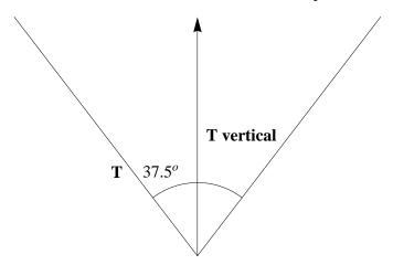
We want to find the tension T such that the vertical component of tension on each side of the strap will be 2.5 N, in other words we want to find T such that :
