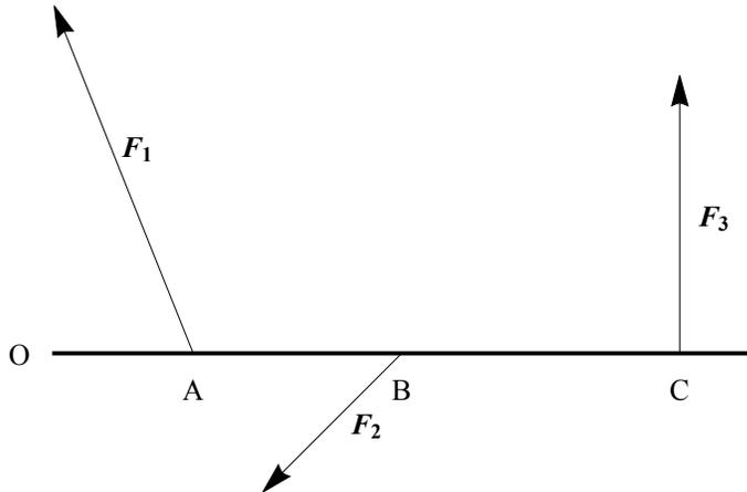
Three forces act on a plank as shown above.  $F_1$  has a magnitude of 40N,  $F_2$  has a magnitude of 20N, and  $F_3$  has a magnitude of 30N. The distances of A, B and C from O are, respectively, 2m, 5m and 9m.  $F_1$  and  $F_2$  make angles of  $45^\circ$  with respect to the plank. Find the torques generated by each force around O, and the direction and magnitude of total torque.
