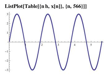
We can also compare the amplitude of the predicted motion with the results of calculation. Our model assumes that x = 0 at t = 0, and that v = 10 m/s at t = 0. This means that at t = 0, all the energy is in the form of kinetic energy, and energy conservation tells us that :
