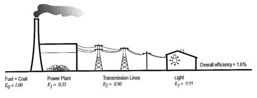
Overall Efficiency for Converting Chemical Energy To Light Energy  $= E_1 x E_2 x E_3 = 0.35 x 0.90 x 0.05 = 0.016$
