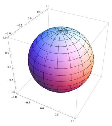
The two sets of braces mean you are plotting over the polar angle,  $\theta$ , from 0 to  $\pi$ , and over the azimuthal angle,  $\phi$ , from 0 to  $2\pi$ .
