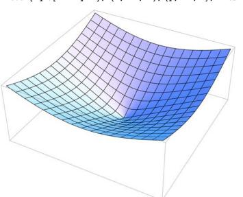
$\texttt{Plot3D[Sqrt[x^2+y^2], \{x, -1, 1\}, \{y, -1, 1\}, \texttt{Filling} \rightarrow \texttt{Bottom]}}$
