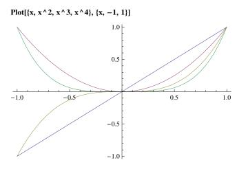
This plots the curves x,  $x^2$ ,  $x^3$ , and  $x^4$  between -1 and 1 on the same set of axes.
